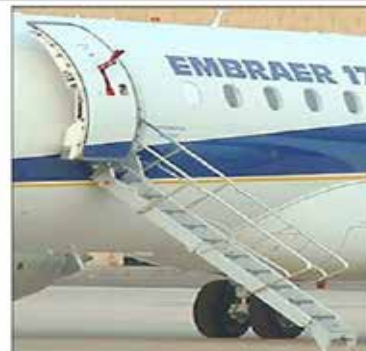
EJet Optional Folding "ladder type" airstair door Additional GSE required to operate door externally
