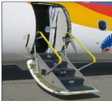
CRJ Standard Integral airstair door Easily operated from ground level
